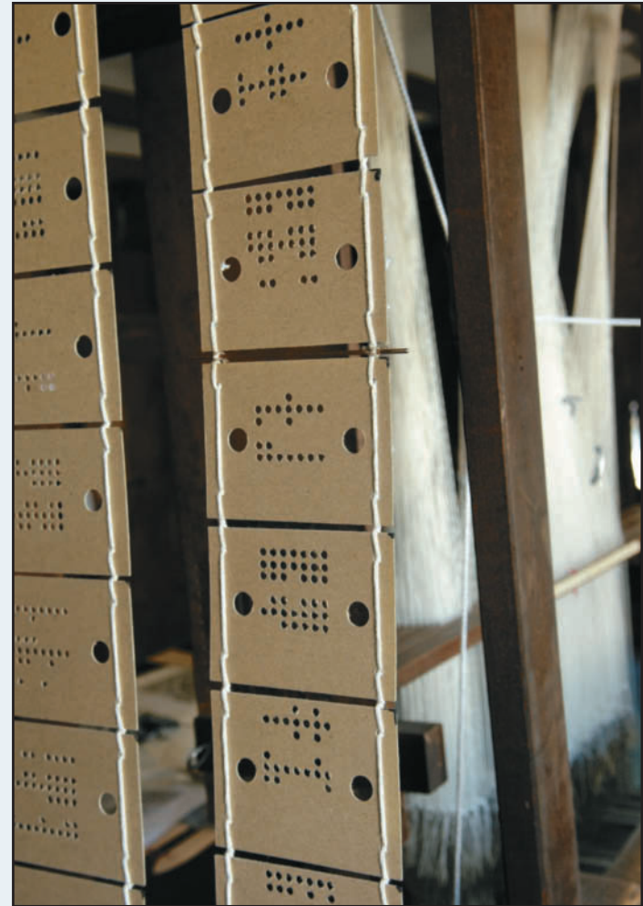
FIGURE 1.1 Punch cards used to create textile patterns in a Jacquard loom.
